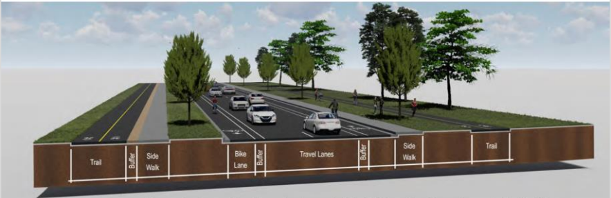
Proposed urban corridor with on-street separated bike facilities, sidewalks, and separated trail facilities.
